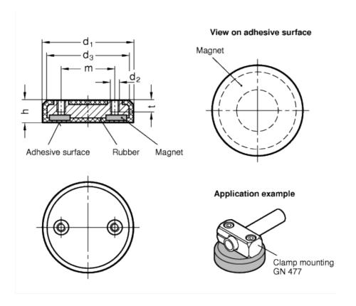
technical informations Specification Disc-shaped, with two female threads, with rubber jacket Steel part, zinc-plated Rubber jacket, Elastomer (TPE), 80 Shore A ≈, black
